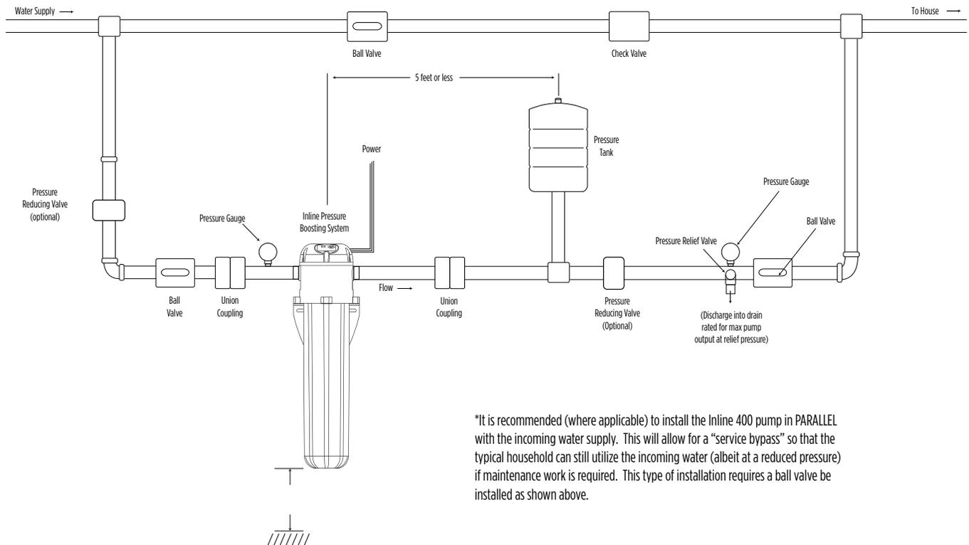
\*It is recommended (where applicable) to install the Inline 400 pump in PARALLEL with the incoming water supply. This will allow for a "service bypass" so that the typical household can still utilize the incoming water (albeit at a reduced pressure) if maintenance work is required. This type of installation requires a ball valve be installed as shown above.
